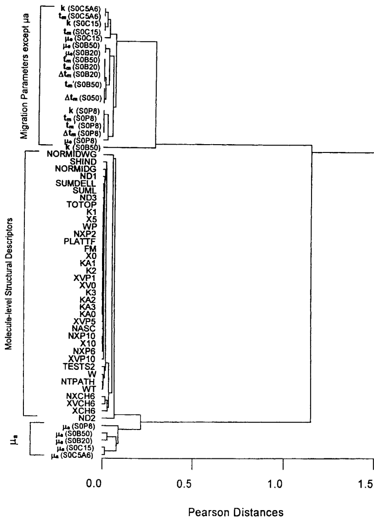
Figure 2. Cluster tree of molecule-level structural descriptors and migration parameters in CZE. The explanation of the molecule-level structural descriptors sees Table 1. Migration parameters obtained under different buffer conditions in CZE: S0B20, S0B50 — SDS 0, borate 20 or 50 mM at pH 10.5; S0P8 — borate 20 mM at pH 8; S0C15 — borate 20 mM, \beta -CD 15 mM at pH 10.5; S0C5A6 — borate 20 mM, \beta -CD 5 mM, 1,3-diaminopropane 6 mM at pH 10.5.
